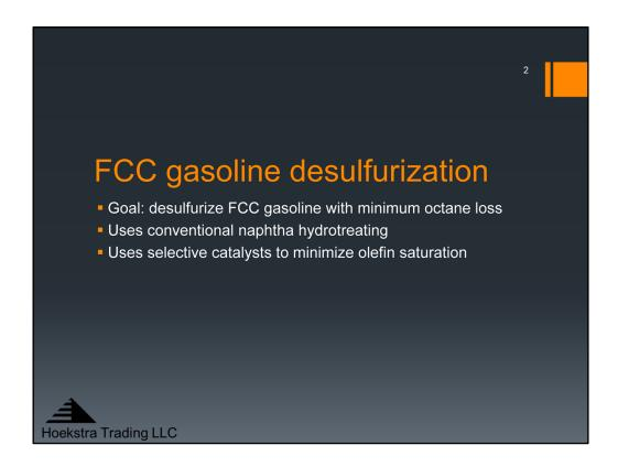
The goal of FCC gasoline desulfurization to desulfurize FCC gasoline with minimum octane loss. The process uses conventional naphtha hydrotreating and selective catalysts to minimize olefin saturation and octane loss.
