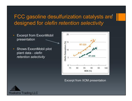
FCC gasoline desulfurization catalysts are designed for olefin retention selectivity.
