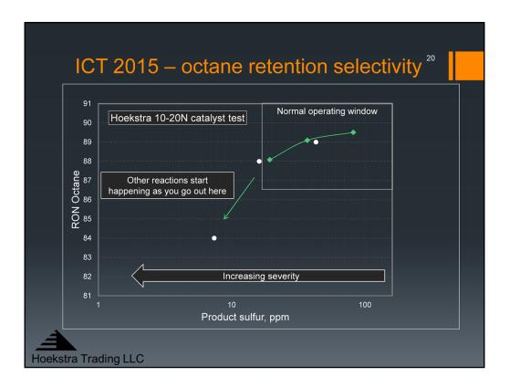
Here we see the other two data points for the more active white catalyst at the medium and high temperatures. With the white catalyst at the high temperature, we made 8 ppm sulfur, and the research octane number went down to 84. For a unit currently making 30 ppm sulfur, that means pushing the unit to 10 ppm comes with a 5 RON octane unit loss on this feed.
