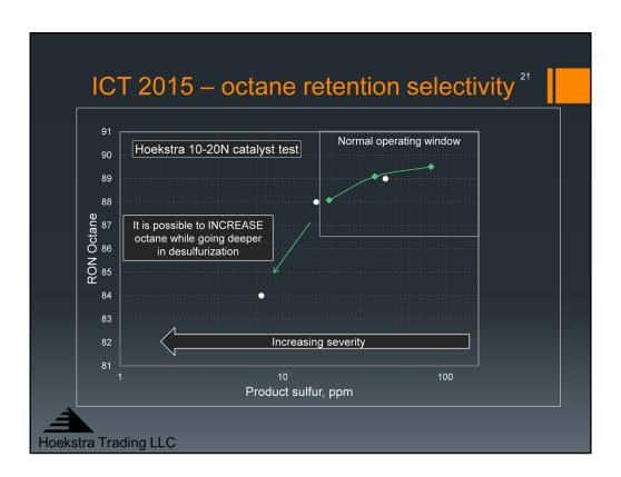
And our detailed data gives insights that suggest it is possible to reduce this 5 octane number loss – in fact, with the right catalyst and unit design, you could increase octane while going deeper in desulfurization.
