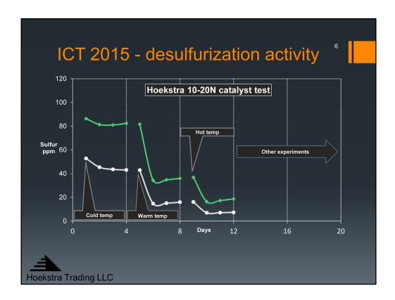
This chart shows product sulfur versus time for the first 12 days of our pilot plant test. Data are shown for two catalysts, one in green and another in white. The test is a 20 day test using a sequence of five test conditions, each test condition is held for four days. The first 4 days are at a low temperature which we call the cold condition, then we increase the temperature to the warm temperature for days 5-8, and then hot temperature for days 9-12.
