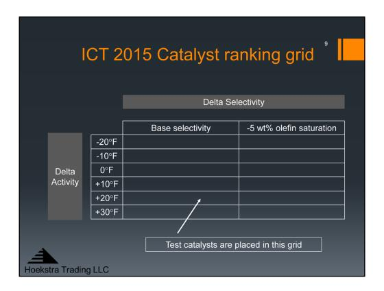
Each catalyst we tested is placed in this grid, based on where its curve fell on the landscape chart. We have vertical tiers indicating delta activity in terms of the equivalent reactor temperature required to get a target product sulfur. We saw two distinct tiers of olefin selectivity. So this ranking grid summarizes the main performance factors important for catalyst selection.
