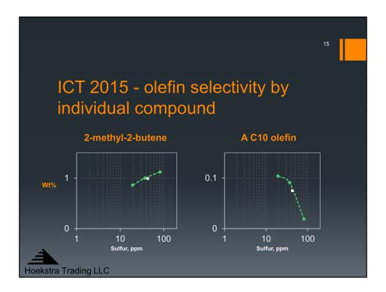
Here is the data for 2-methyl-2-butene, it is a C5-olefin that happens to be present in high concentration in FCC gasolines. And on the right is the chart for a particular C10-olefin.
