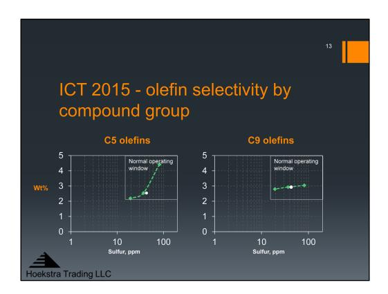
Here I am showing the above data charted on what I called a landscape chart, for the C5 olefins and the C9 olefins (Before we were looking at total olefins). You see the curve for the C5 olefins is steeper, indicating their higher reactivity compared to the C9 olefins on the right.
