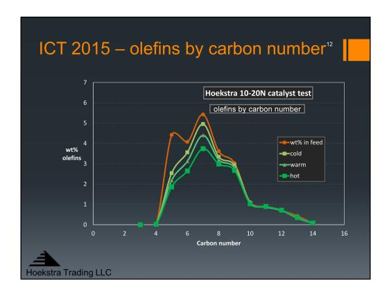
This is the distribution of olefins by carbon number for the feed and those three product samples at the cold, warm, and hot temperatures for the green catalyst. Looking first at the orange curve for the feed, it shows that C5 and C7-olefins are present in the highest concentrations, and the feed contains some olefins all the way up to C14 olefins.
