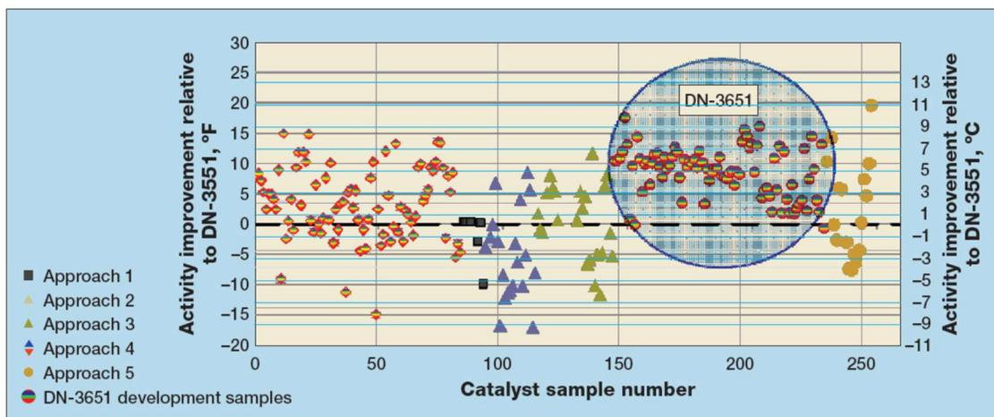
Then Criterion used pilot scale testing to show the activity advantage of the scaled-up commercial catalyst (DN-3651) versus a previous commercial catalyst. The pilot plant shows an activity advantage >10 degrees F which held up in a seven-hundred-hour pilot plant test. This provides the kind of data an engineer needs to drive a catalyst refill decision:
