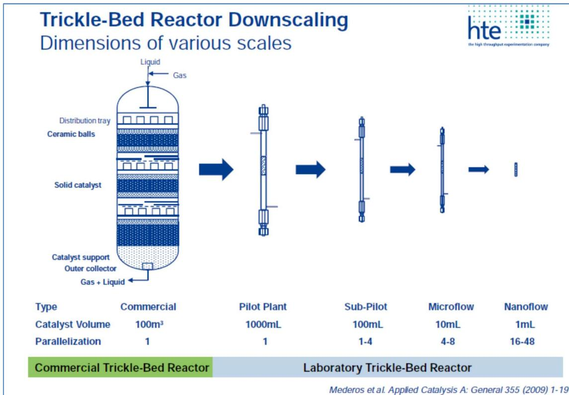
The *nanoflow* unit on the right is ideal for screening hundreds of candidate catalysts per year in catalyst development. The *sub-pilot* units, which are about 50 times that size and typically have 4 reactors per unit, are ideal for evaluating about 10 commercial catalysts per year for the purpose of catalyst selection.
