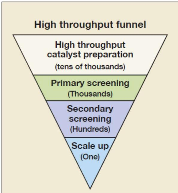
In *catalyst development*, hundreds of candidate catalysts are screened in the primary and secondary screening stages for the purpose of developing an improved commercial catalyst.
